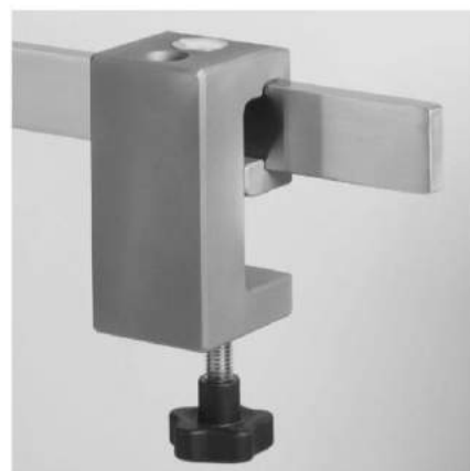
24-799-06 Clamp socket made of light metal, holding width 50 mm, for screw stand \varnothing 16 mm/M10, for rails 25/35 x 8/10 and tubes \varnothing 12 - 35 mm.
