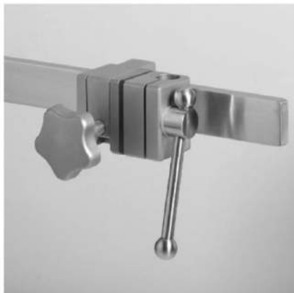
24-799-02 Clamp socket made of stainless steel, for height-adjustable stand \varnothing 16 mm, electrically insulated up to 1.5 kV AC, holding width of 35 mm for rails 25/32 x 8/12 mm.
