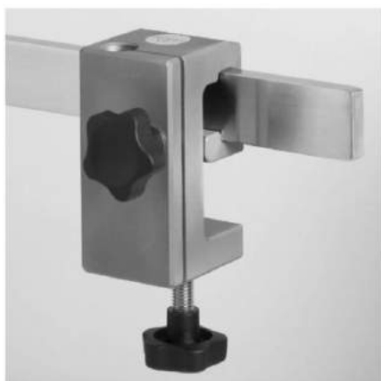
24-799-04 Clamp socket made of light metal, holding width 50 mm, for height-adjustable stand \varnothing 16 mm, for rails 25/35 x 8/10 and tubes \varnothing 12 - 35 mm.
