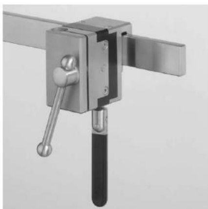
24-799-05 Clamp socket made of stainless steel, for height-adjustable stand \varnothing 16 mm, electrically insulated up to 4.5 kV AC, holding width of 50 mm for rails 25/32 x 8/12 mm.
